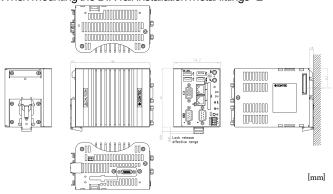
2 To secure this product with the included fittings, use the included screws (M3x7). In other situations, use screws with a penetration depth (L) from the chassis surface to the screw tip of 3 mm or lower.
